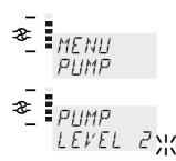
The capacity of the circulating pump is set by adjusting the motor speed Settings: stage / LEVEL 1 ... 4
