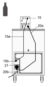
Check to make sure that the line voltage matches the supply voltage specified on the identification plate. Deviations of  $\pm 10$  % are permissible.
