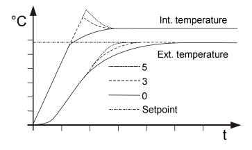
As soon as a co-speed factor is set, it is considered for calculating the control parameters. As shown in the diagram, tuning times become shorter the higher the co-speed factor is, but overshooting can happen in the internal system.
