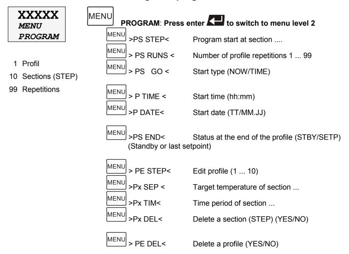
The integrated programmer allows any desired temperature program sequences to be realized. Such a temperature sequence is called profile. A profile consists of individual sections defined by duration (t:) and target temperature. Target temperature is the setpoint (T:), that is achieved at the end of a section. The programmer uses time and temperature difference values within a section to calculate a temperature ramp.
