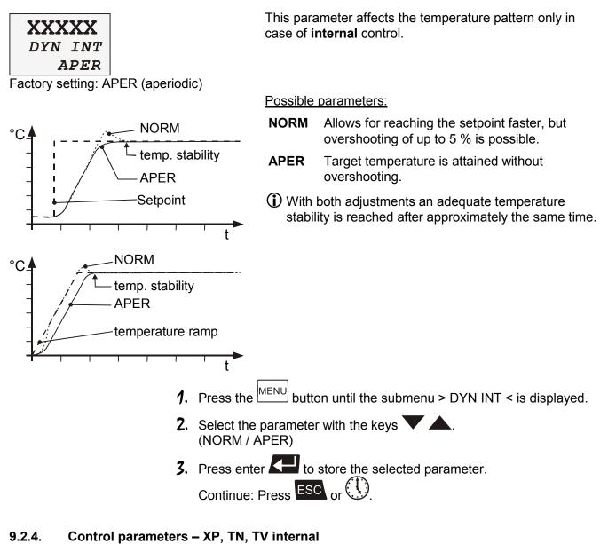
The control parameters preset in factory are in most cases adequate for achieving an optimum temperature pattern for the samples requiring temperature application.
