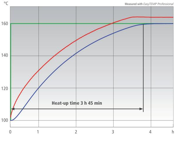
SetpointTemperature in reactor's interiorTemperature in reactor's jacket
