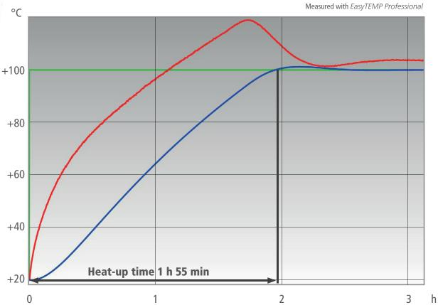
Setpoint Temperature in reactor's interior Temperature in reactor's jacket
