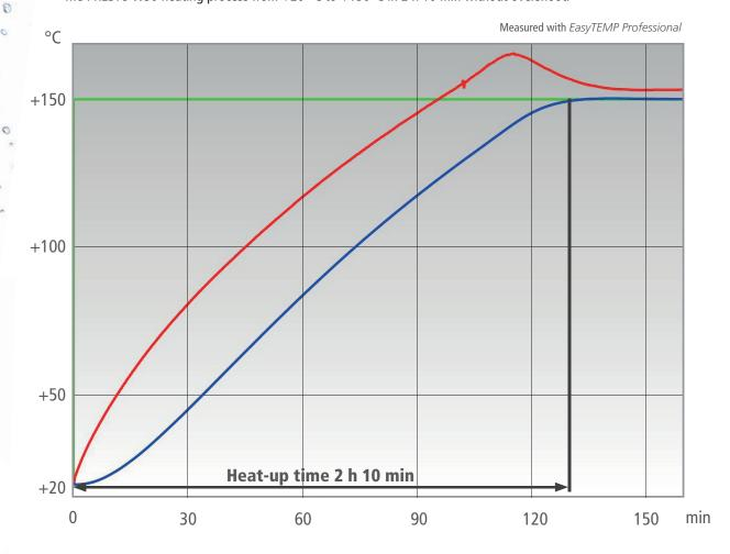
Setpoint Temperature in reactor's interior Temperature in reactor's jacket
