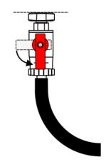
• **Tighten** the **drain tap** after draining the unit and replace the venting grid.
