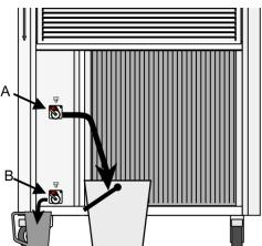
The unit has two drain taps. Both have to be used. First drain the large tank via drain tap A, the drain the remaining liquid via drain tap B.
