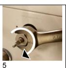
1. Undo the nut (a.f. 8) and remove the hand wheel on the adjustment valve,
