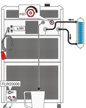
Connect the tubings for cooling the external system to the pump connectors for feed and return (14) on the rear of the recirculating cooler.
