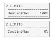
The heating and cooling capacity of the unit are adjustable. 100 % corresponds to the technical specification of the equipment.
