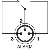
30 W / 40 VA Switching capacity max. Switching voltage 125 V~/max. Switching current 1 A max.
