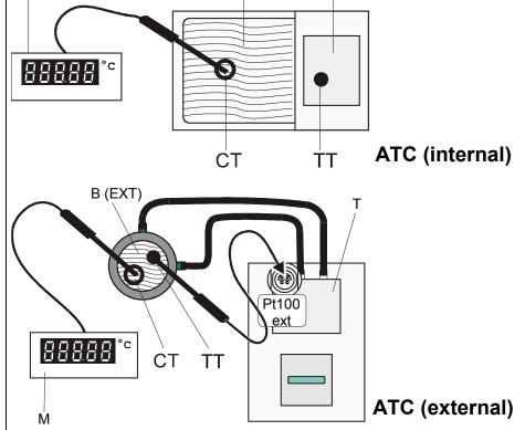
M = Temperature measuring instrument with temperature sensor
