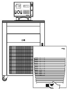
In dusty environments, the refrigerating machine's condenser should be cleaned by vacuuming every 1 to 2 months. The condenser is located behind the venting grid on the front of the unit, which can be taken off by removing the screws.
