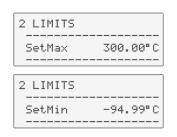
**Set Max / Min–** Maximum and minimum setpoint Restriction of the adjustable temperature range.
