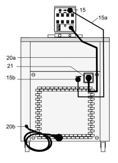
Make sure that the line voltage and frequency match the supply voltage and frequency specified on the type plate.
