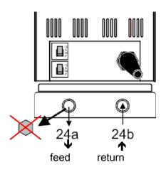
The circulator is used for temperature application to external, closed systems (loop circuit) with simultaneous temperature application in the circulator bath.
