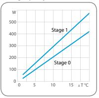
Ambient temperature:  $+20 \degree$ C Return temperature:  $+30 \degree$ C  $\Delta$ T:  $+10 \degree$ C Cooling capacity (stage 1): 300 W
